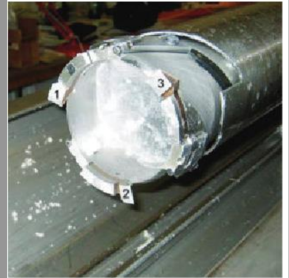
Fig. 14.5. Only in early July, the drill came up with a well sized ice core in the core barrel. The cutter knives, are numbered 1, 2 and 3. Photo: Lars Berg Larsen.
