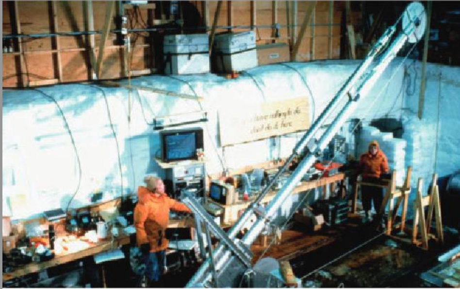
Fig. 10.2 The drill ball, ISTUK is being tilted by a hydraulic pump system.
