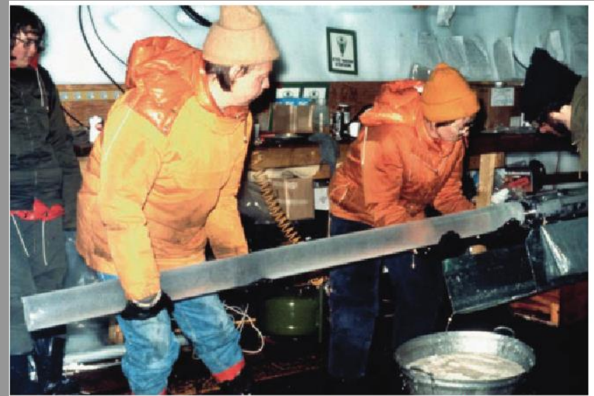
Fig. 10.3 An ice core from great depth is released from the core barrel. Note that it is transparent. The air bubbles are dissolved in the crystal lattice at great pressures. When the ice relaxes at normal pressure they re-appear, but now around micro-parti-
