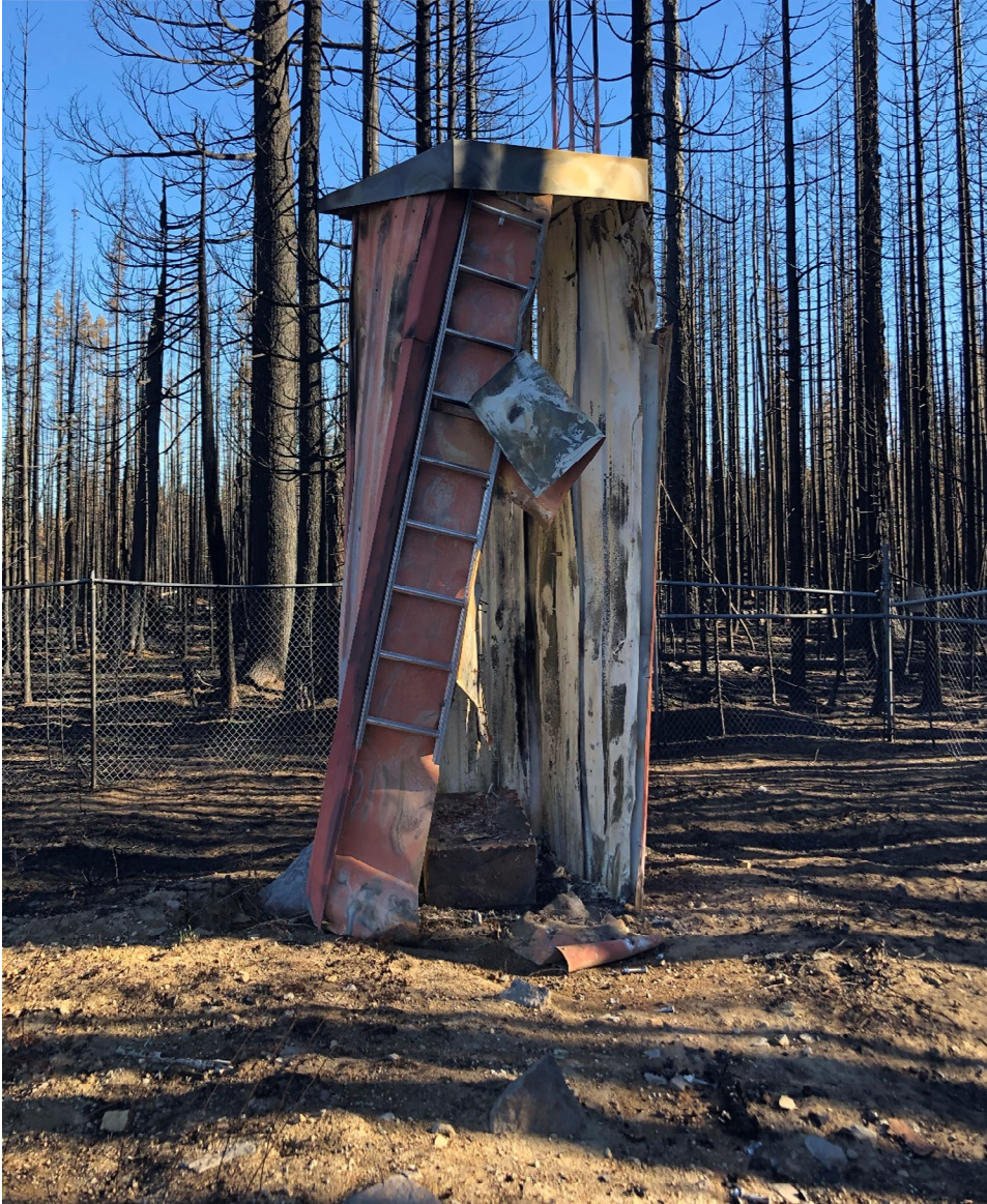
Diamond Lake SNOTEL Burned in Thielsen Fire – 09/09/2020 Klamath Basin
